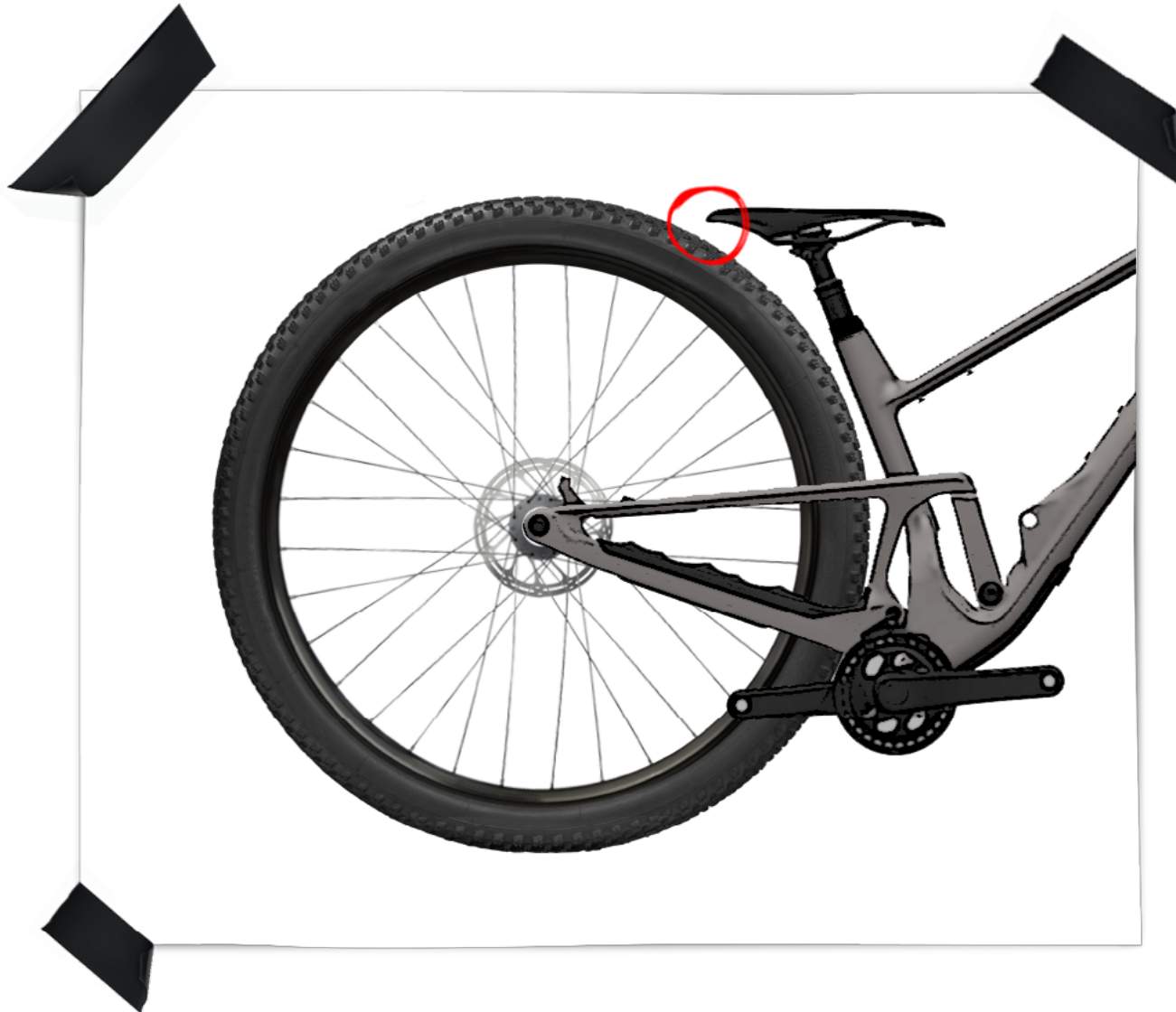
Fig.4 – saddle clearance at full compression
