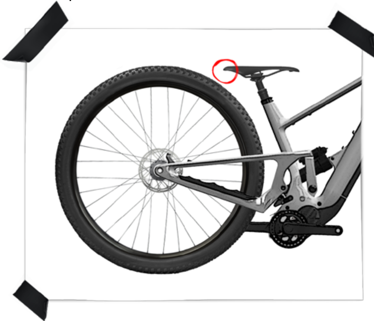
Fig.4 - saddle clearance at full compression
